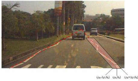
Fig. 8. Region of interest for zigzag detection
