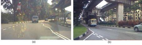
Fig. 7. Possible zigzag marking scenarios (a) Most common with solid marking preceding zigzag (b) Case with dashed marking at cross road preceding zigzag
